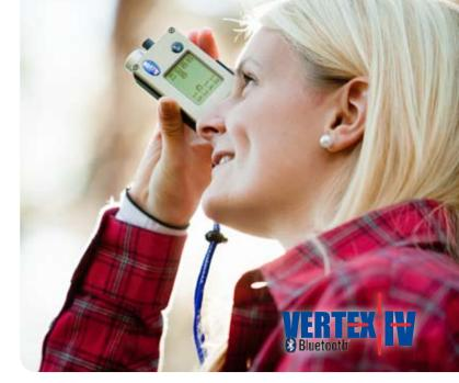
The Vertex instrument works great to measure radius in sample plots, it simplifies the job and ensures a much more accurate result. With the built in BAF function you are able to be at the tree and determine its minimum diameter to be included into the point. The BAF function allows you to prism cruise on track with thick underbrush that you normally could not do using a standard prism.
